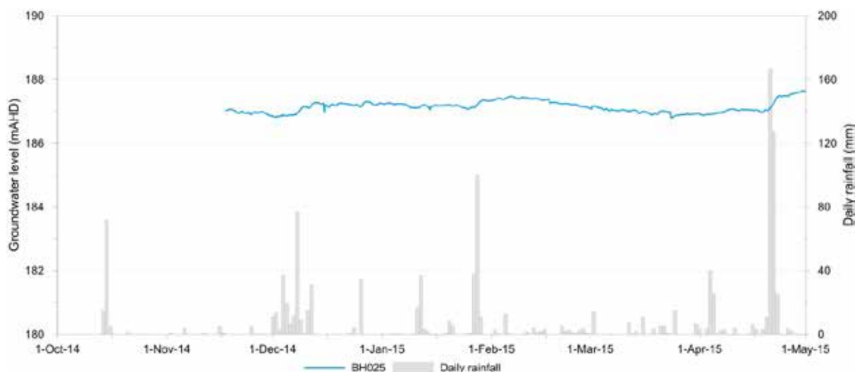
Figure 3.19 BH025 (shale) groundwater level and daily rainfall (Turramurra station)
