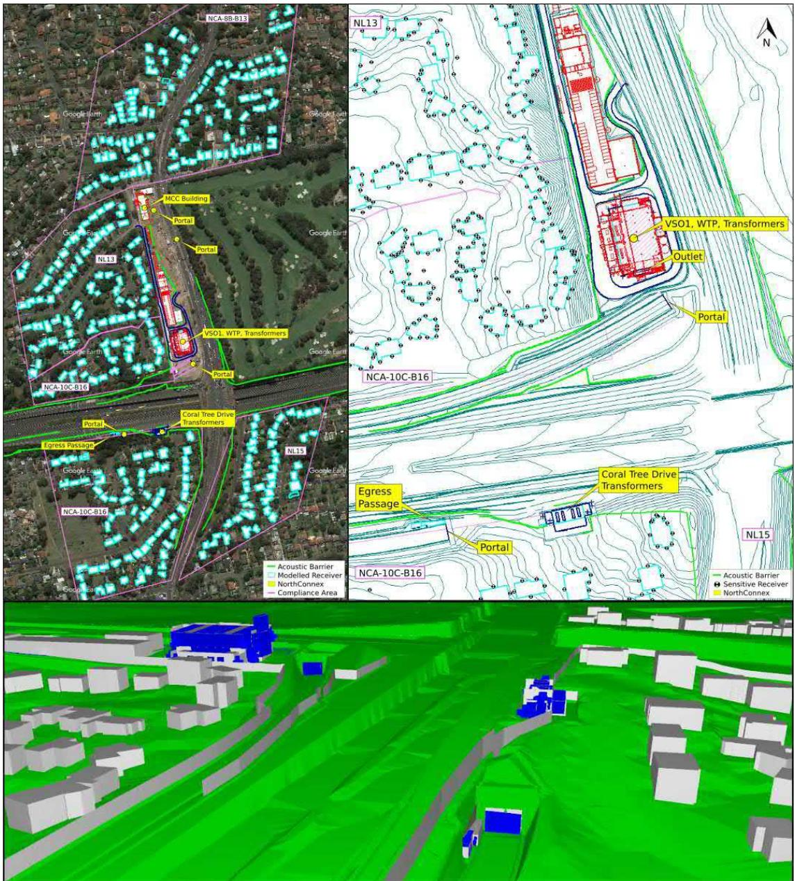
**Figure 9-11 Recommended Noise Wall (in red) along the Western Boundary of the Southern Compound**
