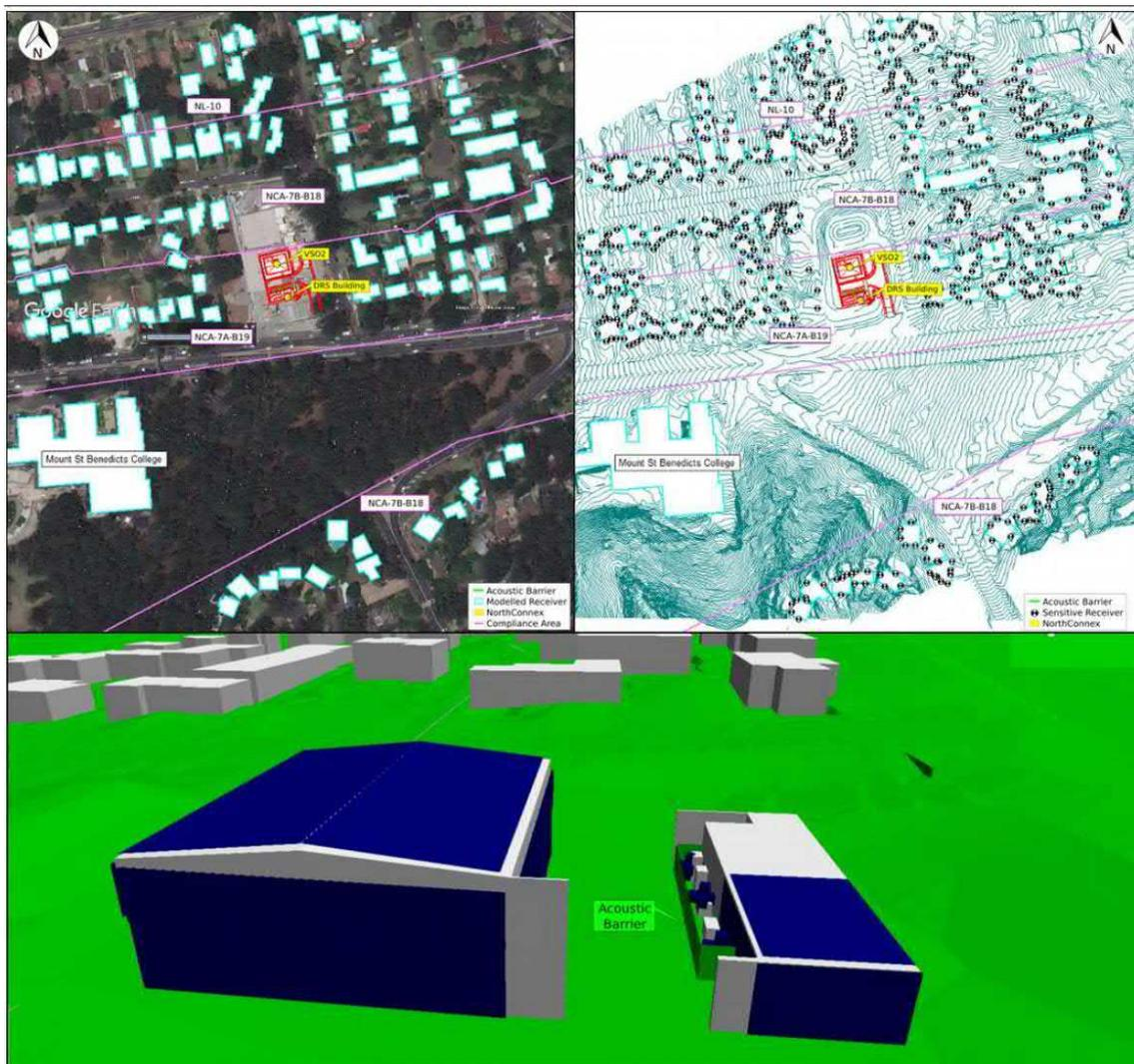
Figure 9-5 presents a 3-D wire-model prepared using the acoustic model to illustrate the relevant areas of the VSO2 building and nearest sensitive receptors.
