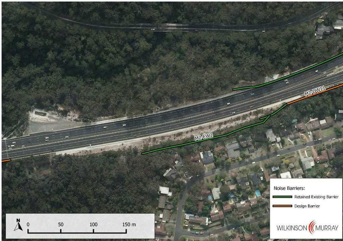
The target barrier exceeds 8m high whilst the assessed barrier is 4.2m high. As noise barriers more than 8m high are considered visually unacceptable, the target barrier has been discarded. As the initial barrier design is 4.5m high, the 4.2m high barrier has been discarded. Based on this, there is no need to modify the height of the exiting noise wall. Further details can be seen in Table 6-27 and Figure 6-34.
