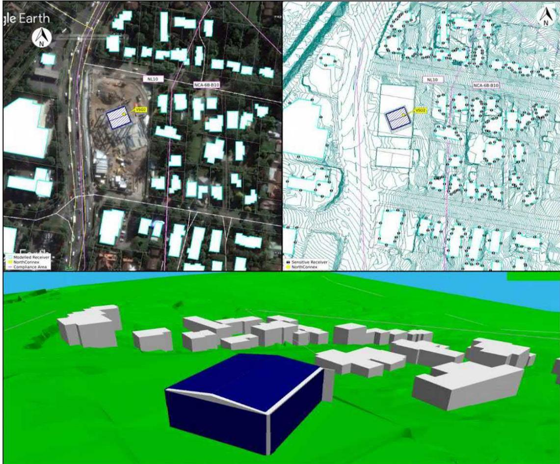
Figure 9-8 presents a 3-D wire-model prepared using the acoustic model to illustrate the relevant areas of the VSO3 building and nearest sensitive receptors.
