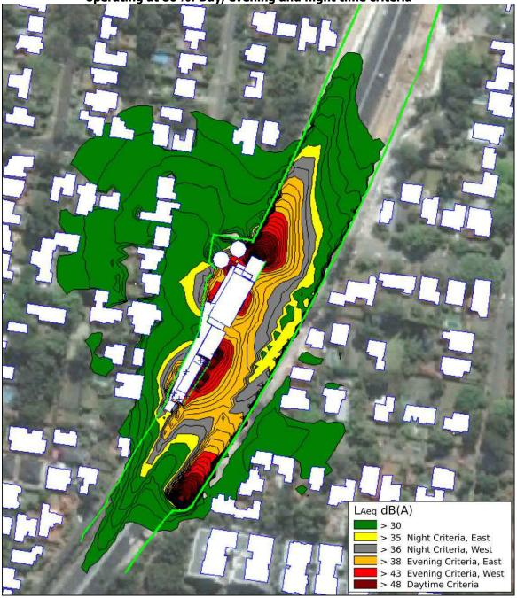
Compliance with the acoustic assessment criteria is predicted at all sensitive receivers in the surrounding area of VSO4, based on the building design, equipment performance, and attenuator performance items detailed in Appendix K:
