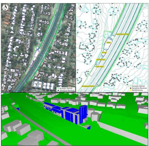
Figure 9-2 presents a 3-D wire-model prepared using the acoustic model to illustrate the relevant areas of the VSO4 building and nearest sensitive receptors.
