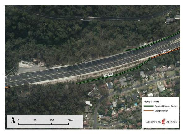
The target barrier exceeds 8m high whilst the assessed barrier is 4.2m high. As noise barriers more than 8m high are considered visually unacceptable, the target barrier has been discarded. As the initial barrier design is 4.5m high, the 4.2m high barrier has been discarded. Based on this, there is no need to modify the height of the exiting noise wall. Further details can be seen in Table 6-27 and Figure 6-34.
